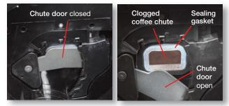
Once bean container lid is removed, the coffee chute door will open. This allows for easy access to the ground coffee chute.
