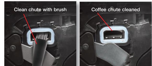
Using the angled cleaning brush, remove any residue from the ground coffee chute and sealing gasket.
