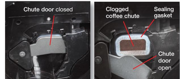
Run a Grind & Clean Cycle and the coffee chute door will open. This allows for easy access to the ground coffee chute.
